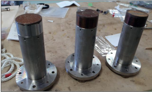
Fig. 13 HY-80 witness rods ready for installation.
