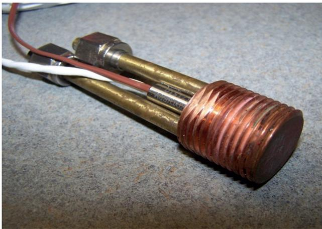
Fig. 7 Medtherm calorimeter.
