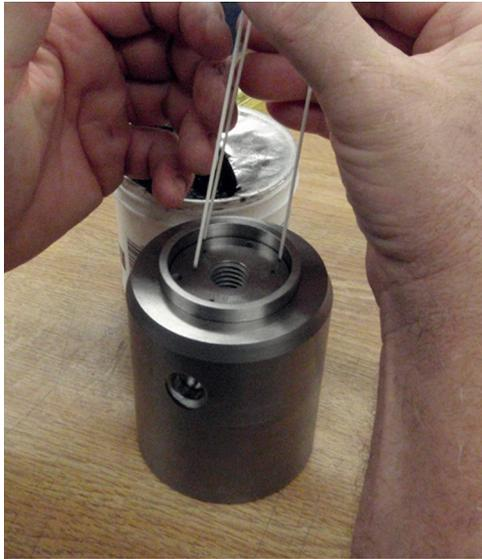
Fig. 10 Insertion of thermocouples into a test article.
