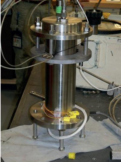
Fig. 15 Static leak check and dynamic response testing.
